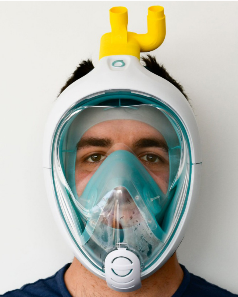
Italian company Isinnova demonstrating their 3D printed adapter converting snorkeling masks into ventilator masks. Photo courtesy of Isinnova.
